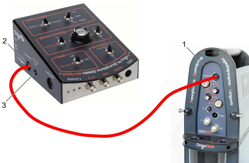
1. Reference electrode                      2. Working electrode                      3. Auxiliary electrode
