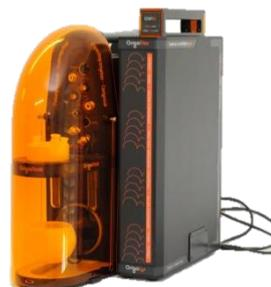
**FRA Unit Impedance 10  $\mu$ Hz – 5 MHz**
