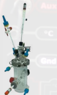
Corrosion Cell supply
